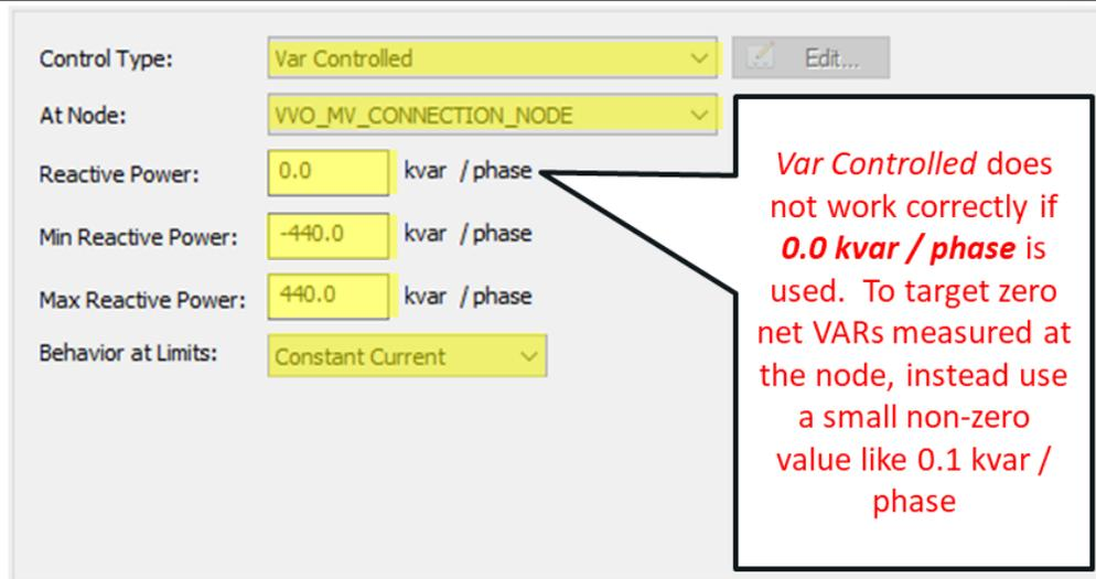
Figure 5: CYME Power Factor Control Used to Simulate VVO Feeder Var Mode
